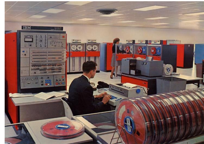
IBM CP-40 mainframe – the first system invented for server virtualization
